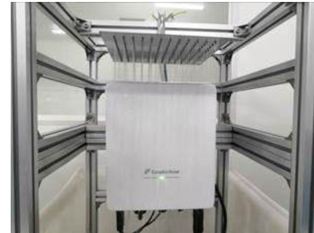
Showering test @ Powering
